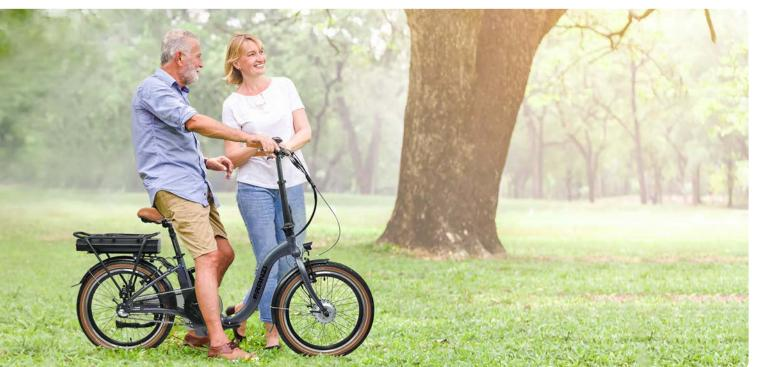
The low entry models FRANZI® in the color "titanium" matt and LOTTE® Mod. 2024 in the color "warm-grey" have a front motor. This is specially adapted to the wheels and thus allows a practical coaster brake in addition to the front wheel brake.
